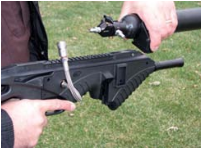
The FN 303 operates off a high-pressure, low-volume compressed air tank filled from a SCUBA tank.
