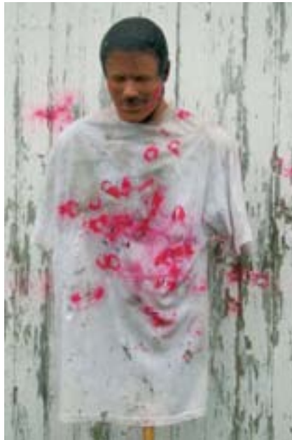
The FN 303 easily put projectiles on a full-size mannequin from the maximum engagement range, and it did it at the rapid-fire rate of one shot per second.
