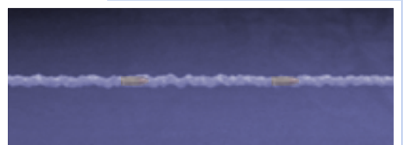
› A 9mm projectile passes through an entire block of gelatin, causing increased risk of overpenetration and collateral damage.
